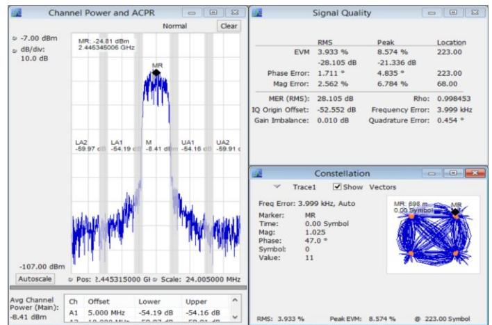
SignalVu-PC Option SV26 enables quick, standards-based transmitter health checks on APCO P25 signals. The following image shows a Phase II signal being monitored for anomalies with the spectrum analyzer while performing transmitter power, modulation and frequency measurements.
