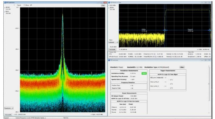
Sophisticated WLAN measurements are easy. On the displayed 802.11g signal, the spectrogram shows the initial pilot sequence followed by the main signal burst. The modulation is automatically detected as 64 QAM for the packet and displayed as a constellation. The data summary indicates an EVM of -33.24 dB RMS, and burst power is measured at 10.35 dBm. SignalVu-PC options are available for 802.11a/b/j/g/p, 802.11n and 802.11ac to 40 MHz bandwidth.
